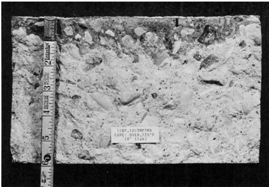
Fig. 1. Fracture surface of surface-impregnated slab. Dark area at top is polymer-impregnated zone. Monomer is MMA.
